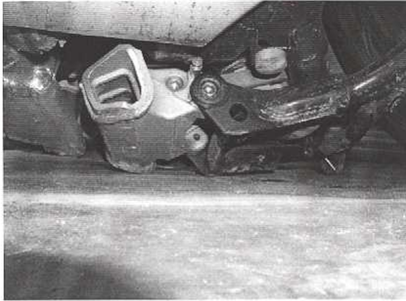
Photo 3 – Separated crossmember and centerstand dragging on ground
