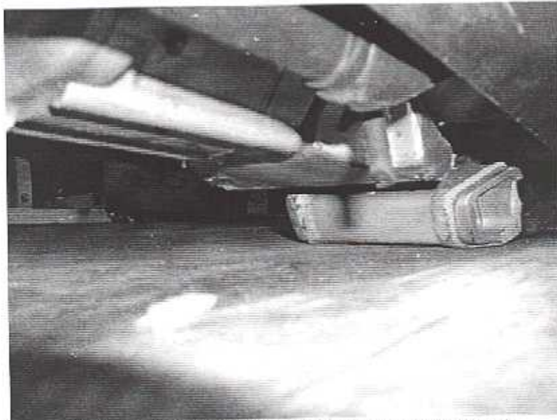
Photo 2 – Separated crossmember dragging on ground
