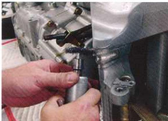
3. Use acetone or an equivalent to clean any grease, oil, or remaining dirt from the welding zone.
