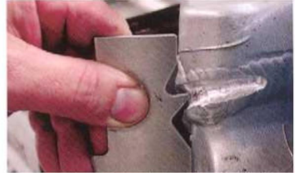
Measure the grind depth along the length of the grind with the Grind Depth Gauge as pictured.
