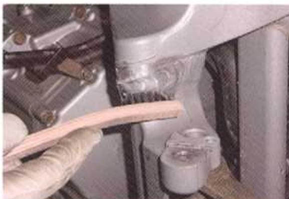
2. **The 2nd weld acts as a shelf for the remaining horizontal welds.** The center of this shelf weld must be located on the edge of the production weld (50% on the production weld, 50% on the casting).
