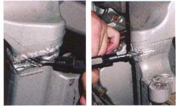
Make sure you grind on both sides of the cross-member and to the full length of the grind mark.
