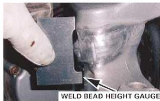
5. **Using additional welding rod**, run one continuous wash bead over all the horizontal beads, making sure to cover the start/stop point of all the beads by at least 2/3 bead overlap.
