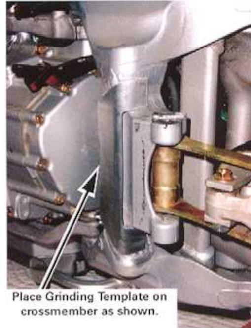
1. With the Grinding Template in the correct position, mark along the edges of the template as shown. Make sure you mark the entire length of the template. **DO NOT mark past the edges of the template.**
